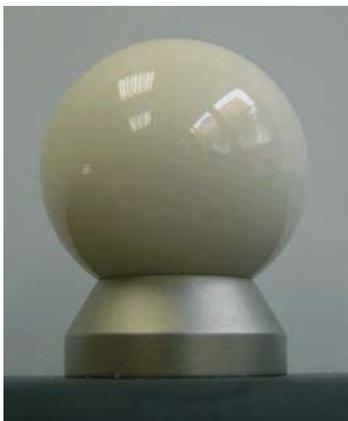
The ceramic probing spheres of  $\varnothing 30$  mm is standard (other diameters are possible) are fixed mechanically in a tapered seating such that adhesive cannot influence the sphere position in a negative way.
