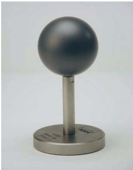
Sphere standard with diffuse reflecting surface
