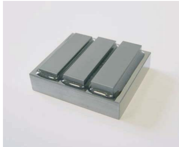
2-Stepped standard with diffuse reflecting measuring faces
